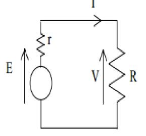
The source resistance is dependent purely on the source and is a constant, as is the source emf. Thus only the load resistance R is a variable.
