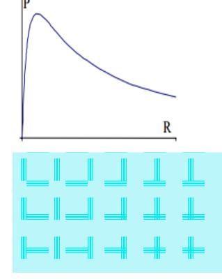
It is to be noted that when maximum power is being transferred, only half the applied voltage is available to the load, and the other half drops across the source. Also, under these conditions, half the power supplied is wasted as dissipation in the source.
